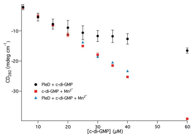
**Figure 7.** Plot of the CD signal at 282 nm of samples containing increasing amounts of c-di-GMP in the presence of 10 μM PleD (monomer) (circles) or 2.5 mM MnCl<sub>2</sub> to the samples containing 25, 30, 35 and 40 μM c-di-GMP and 10 μM PleD yields the same CD signal (triangles) of the manganese-alone samples. Experimental conditions were as follows: 20 mM Tris-HCl, pH 8, 100 mM NaCl, 10 mM MgCl<sub>2</sub>, 1 mM BeCl<sub>2</sub> and 10 mM NaF. The assays were performed in triplicate.
