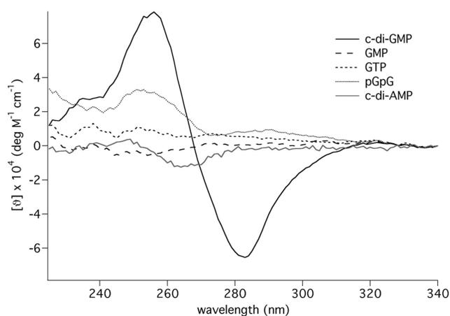
**Figure 5.** CD spectra of the nucleotides involved in c-di-GMP turnover. The nucleotides were analyzed at the concentration of 15  $\mu\text{M}$  at 10°C in 50 mM Tris-HCl, pH 7.5, 150 mM NaCl, 10 mM  $\text{MgCl}_2$  and 2.5 mM  $\text{MnCl}_2$ . The spectrum of cyclic-di-AMP is also shown to compare the behavior of the two cyclic dinucleotides (c-di-GMP and c-di-AMP).
