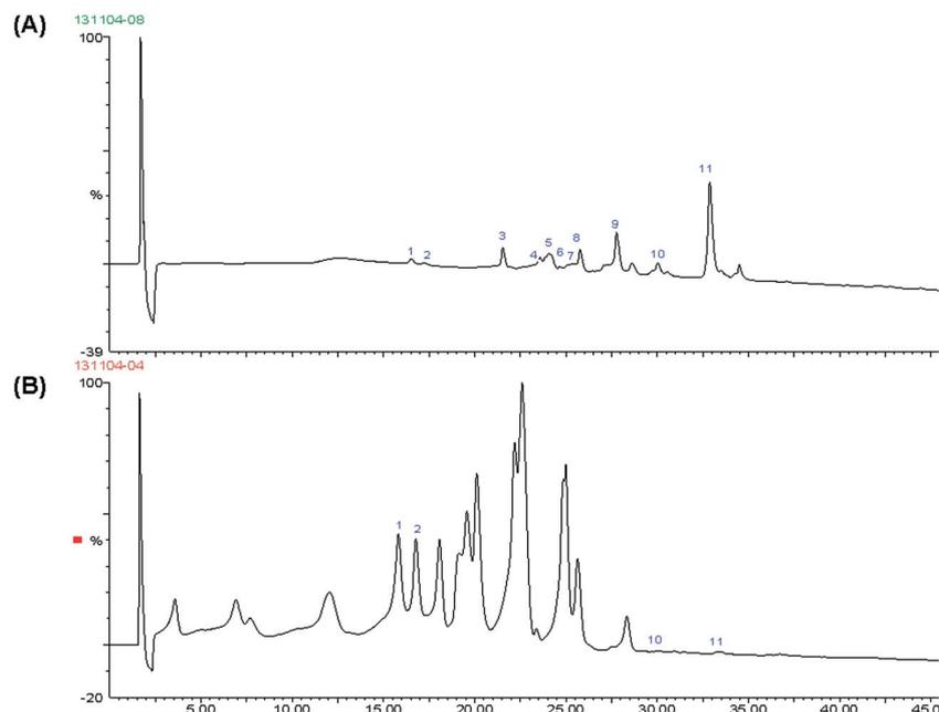
Fig. 1 HPLC-DAD chromatograms monitored at 280 nm of (A) *Artemisia campestris* aqueous extract (ACAЕ) and (B) standard mixture.
