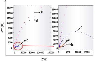
Figure 2. Nyquist plots of developed influenza A viral biosensor. a.Plain AuSPE, b. AuSPE/graphene-AuNp, c. AuSPE/graphene-AuNp/fetuin d. AuSPE/graphene-Α. AuNp/fetuin A/N, e. AuSPE/graphene-AuNp/fetuin A/N/PNA lectin. The EIS procedure was set to measure the electron transfer resistance in the frequency range of 0.1 Hz –10 kHz at potential of 0.1 V and 10 mM  $K_3[Fe(CN)_6]/K_4[Fe(CN)_6]$  (in pH:7.4, 0.1 M PBS) was used as a redox probe.
