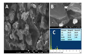
**Figure 1.** A), B) SEM images of graphene-Au nanocomposite and C) EDS results of graphene-Au nanocomposite.
