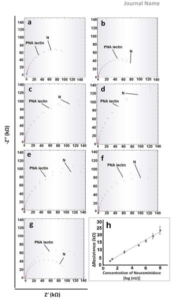
**Figure 3.** Nyquist plots of different concentration of N; a)10<sup>-8</sup>U/mL, b)2x10<sup>-8</sup>U/mL, c)10<sup>-6</sup>U/mL, d)10<sup>-5</sup>U/mL, e)10<sup>-3</sup>U/mL, f)10<sup>-2</sup>U/mL and g)10<sup>-1</sup>U/mL; which were used for calibration graph and h)the calibration graph of developed electrochemical influenza virus A biosensor.
