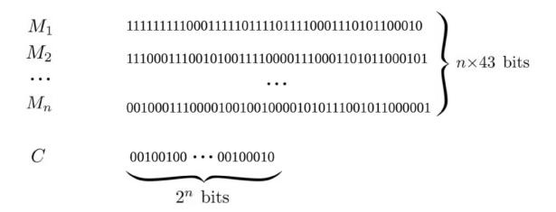
Figure 2. Binary representation for an EA solution.
