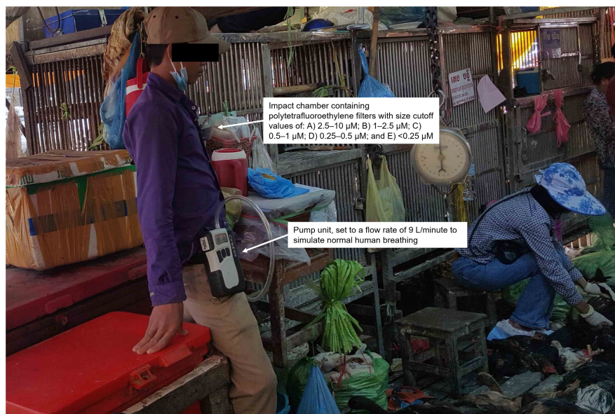
FIGURE 1 A live bird market vendor wearing a personal aerosol impact sampler during the study
